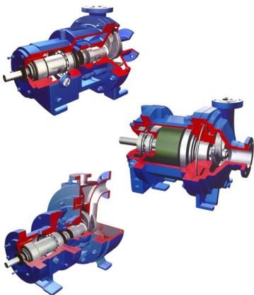
**Truflo** offers component interchangeability between our own products. The **DAP**, **DSP**, and **MAP Series** all use many of the same parts. The DAP and MAP Series both use the same casing. The DAP and DSP Series share the same impeller, power frame and end cover.
